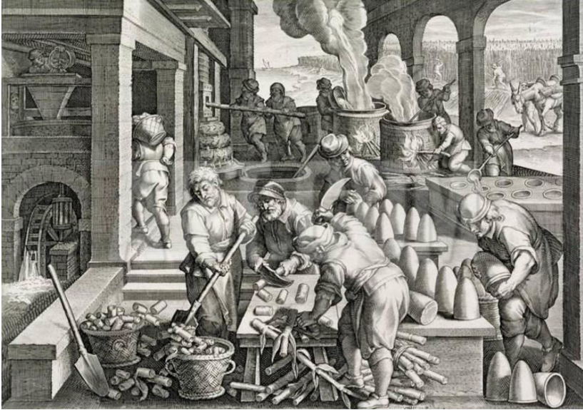
2. A sugar mill, illustrating the production of sugar loaves or cones. Design by Jan van der Straet for a series of prints, “Nova reperta”, (Antwerp, c.1590) showing recent inventions.
